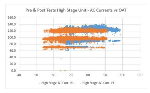
It's clearly visible that in post-treatment measurements, the difference between maximal and intermediate Amp-levels became smaller, and levels themselves – more consistent. While this Iced Cold effect requires additional analysis / investigation, it might be indication that high stage compressor operates after Iced Cold treatment "not as hard as before" treatment, which could be translated into extended equipment lifetime.
