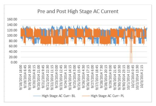
While sufficient Amps and/or Amp-hours decrease wasn't detected for High-stage compressor, the three Amps levels for current's variations became significantly different in post-treatment, than they were in pre-treatment. The difference is presented below:
