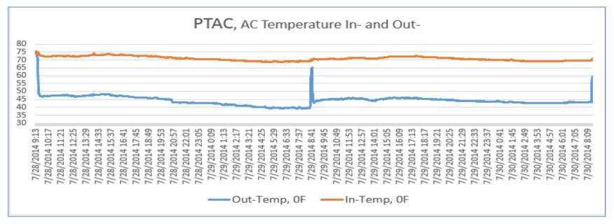
Chart presents two days of Lobby's PTAC unit operations - before and after IceCold treatment. The mode of unit's operation in both days - operating consistently loaded.
