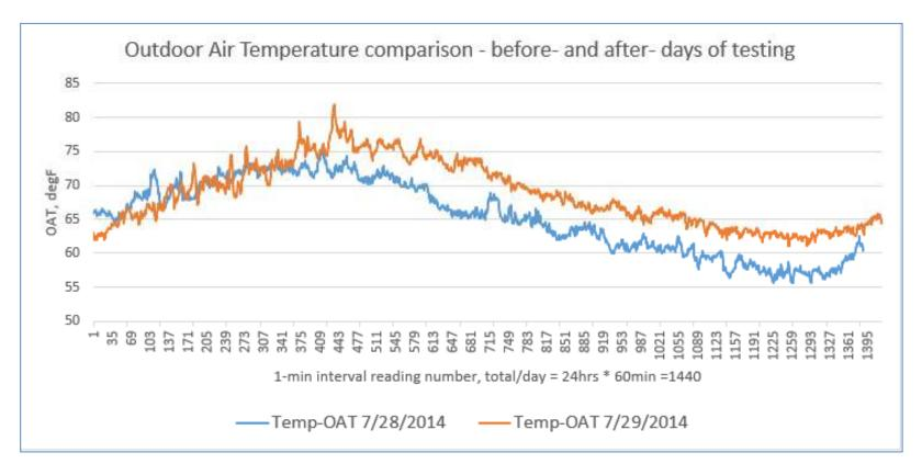
Comparison of weather-normalized energy usage is important for rproper esults interpretation. In this case, it should be noted that after-treatment AC current data was collected at 35% warmer outdoor conditions (35% more Cooling Degree Days)
