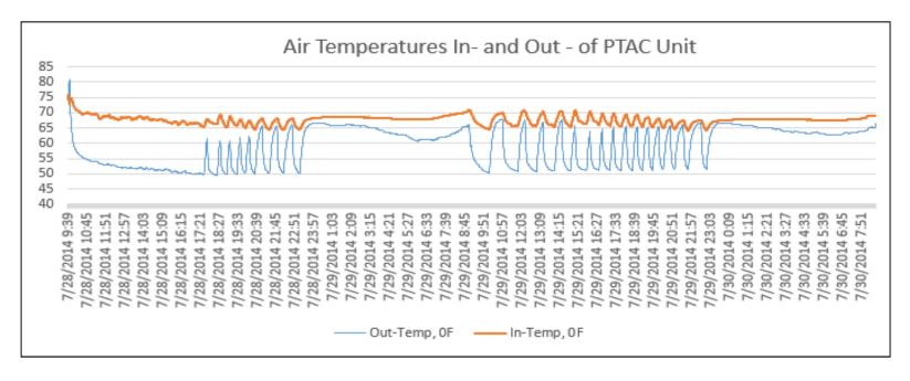
In both analyzed days PTAC unit operated between about the same In- and Out- temperatures
