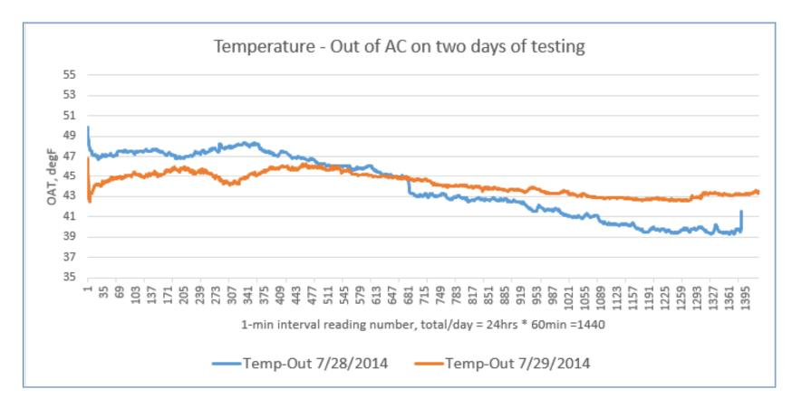
Temperature of air leaving PTAC unit was in average the same in two days of testing. In after-treatment day it was observed colder air leaving PTAC in the morning, and warmer on evening
