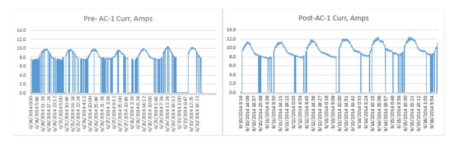
Charts above compare electric Currents drawn by AC-1 unit before and after IceCold treatment. Visual comparison indicates larger Amperage and longer operational time with after-treatment conditions. However, as earlier charts indicate, comparison shouldn't be performed of "intuitive, visual" basis.
