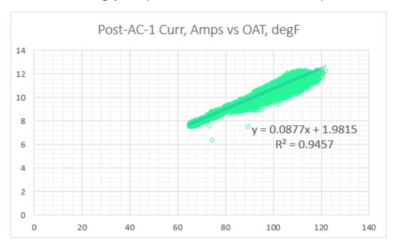
Chart above represents relationship between electric current drawn by AC unit and ambient temperature.
