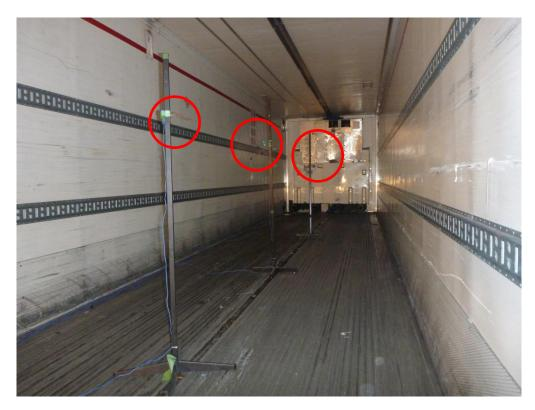
Figure 12. Position of the three thermocouples in the middle of the trailer
