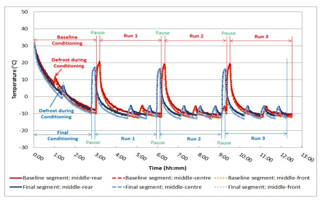
Figure 15. Trailer interior temperature variations during the tests: sensors in the middle of the trailer
