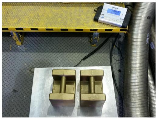
Figure 10. Scale verification using calibration weights
