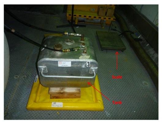
Figure 5. Installation of the portable fuel tank
