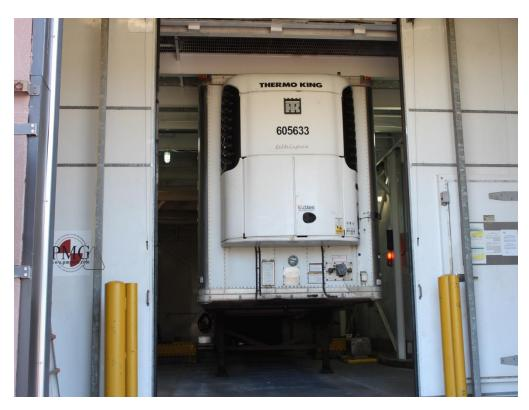
Figure 3. Refrigerated trailer and refrigeration unit in the environmental chamber
