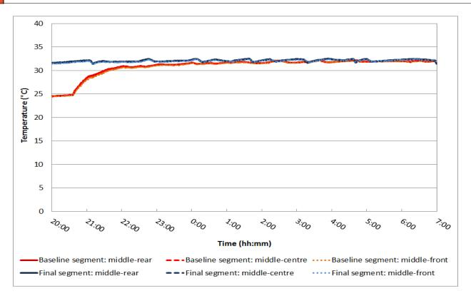
Figure 13. Trailer interiror temperature variations during soaking
