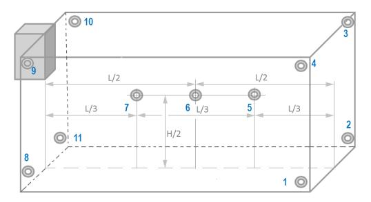
Figure 11. Position of the thermocouples inside the trailer
