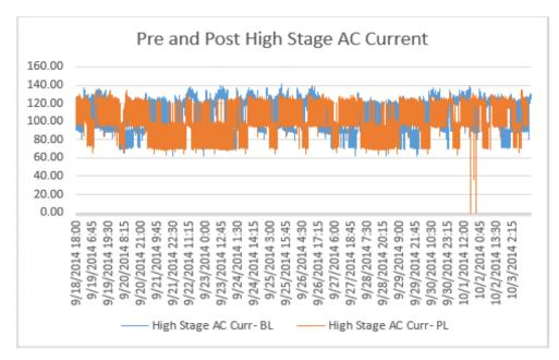
While sufficient Amps and/or Amp-hours decrease wasn't detected for High-stage compressor, the three Amps levels for current's variations became significantly different in post-treatment, than they were in pre-treatment. The difference is presented below:
