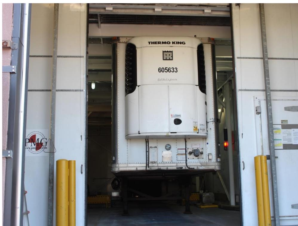
**Figure 3. Refrigerated trailer and refrigeration unit in the environmental chamber**
