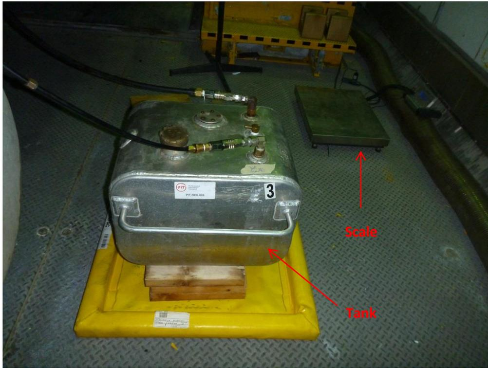
Figure 5. Installation of the portable fuel tank
